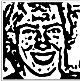
Fig. 6.23. The sign of the shape index divides the image into predominantly positively ( white ) and predominantly negatively ( black ) curved areas. Such images typically look like “sketches”, even more so when the black areas are skeletonized
